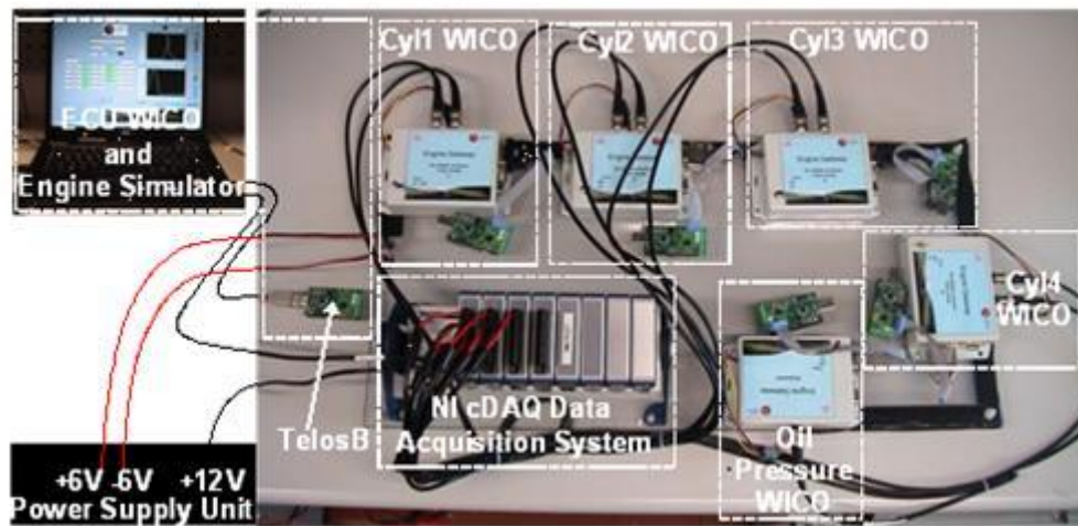
Figure 7: Engine WICOs Experimental Setup: the acquisition board, the 6 WICOs and the ECU implemented on a Laptop
